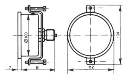
Case and rim: AISI 304 stainless steel. Fully sealed.
